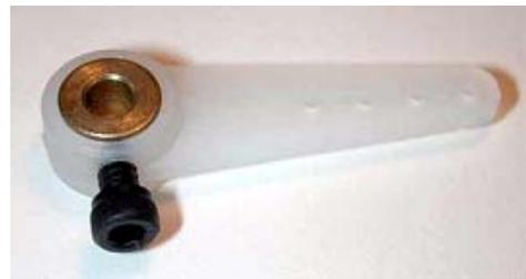
Rudder Arm with Insert (Photo #13)
