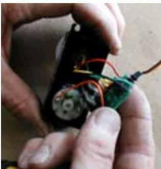
Removing Circuit Board (#16)
